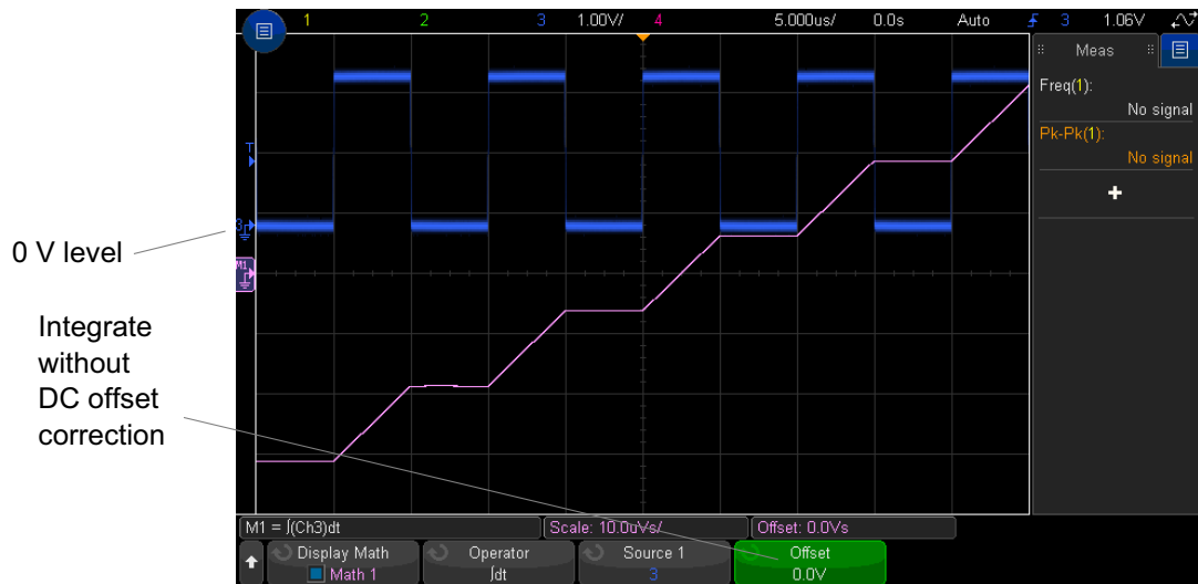
Figure 9 Integrate Without Signal Offset
