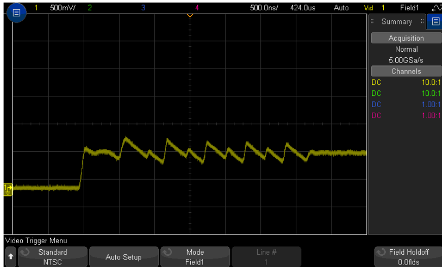
Figure 32 Triggering on Color Field 1 Alternating with Color Field 3
