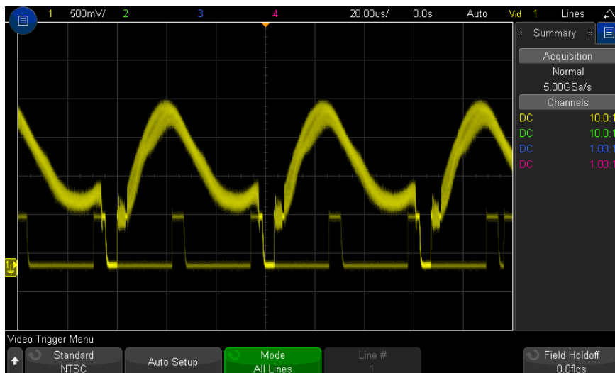
Figure 29 Triggering on All Lines
