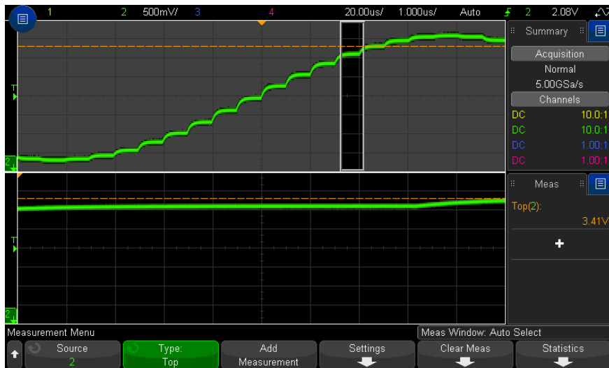
Figure 47 Isolating area for Top measurement
